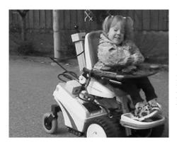
Sara also started out with an Akka. Now she's no longer limited to following a taped line. She can move anywhere in her electric wheelchair. She uses four switches. One to go forward, one to go backwards, one for turning right and one for turning left. It's also possible to move the seat up and down with help of the switches.
