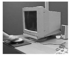
A special keyboard called "Octopus" is designed so that the computer can be controlled by switch guiding. You press a button that you have attached to the Octopus and something happens.
